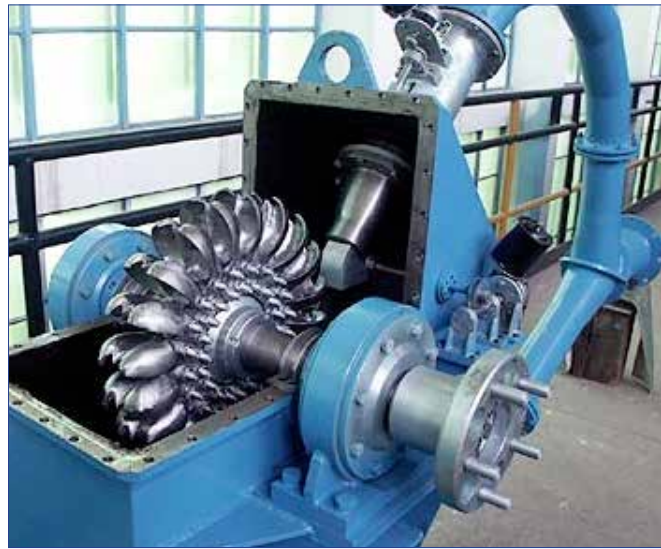
A Pelton wheel turbine showing the rows of buckets around the rim and the 2 nozzles which direct the water at the wheel.
